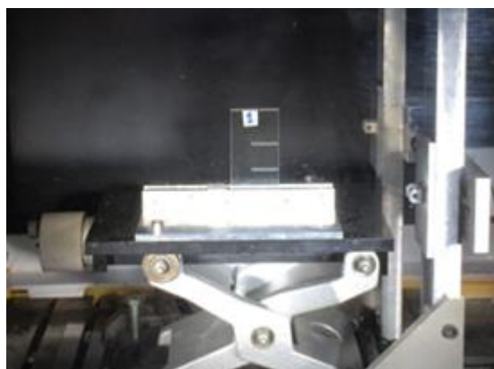
Figure 1: KW-type impact tests. View of the double notched plate in a closed chamber with the support table. The projectile hits the edge of the plate from the right side.
