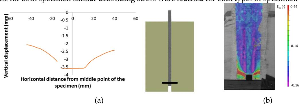
**Figure 8.** (a) debonding starting at the bottom of the specimen, (b) compression at the interface before debonding
