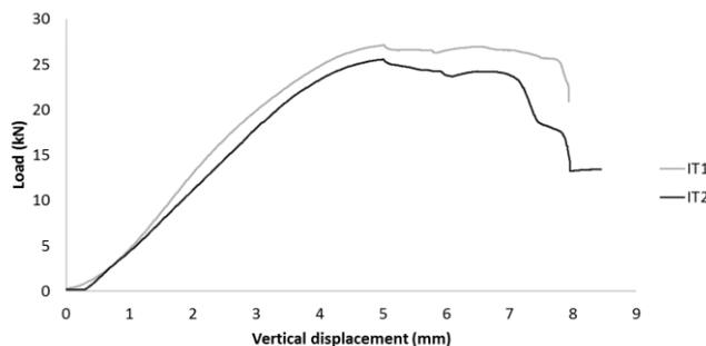
**Figure 7.** Load-displacement curves of inserted type bond test
