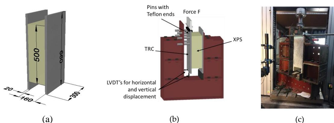
**Figure 1.** (a) specimen geometry and dimensions in mm, (b) schematic presentation of the double-lap shear test, (c) picture of double-lap shear test
