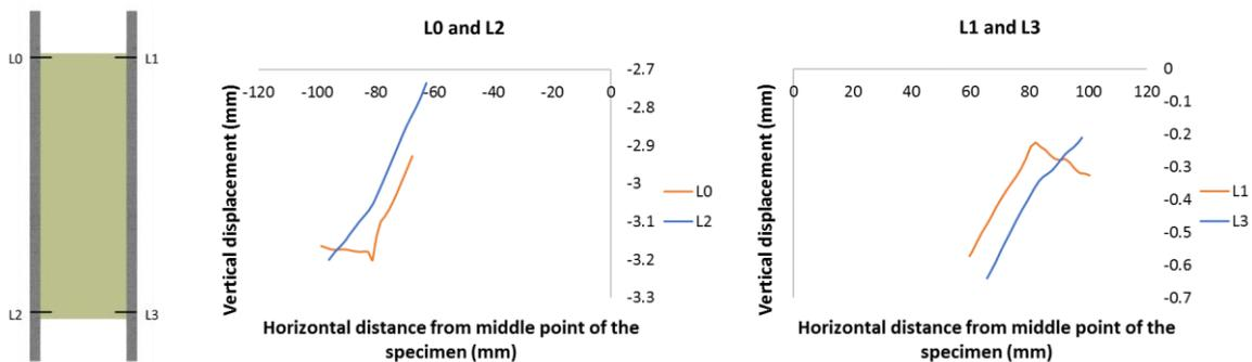
Figure 5. initiation of debonding (line L0) at a load of 22kN
