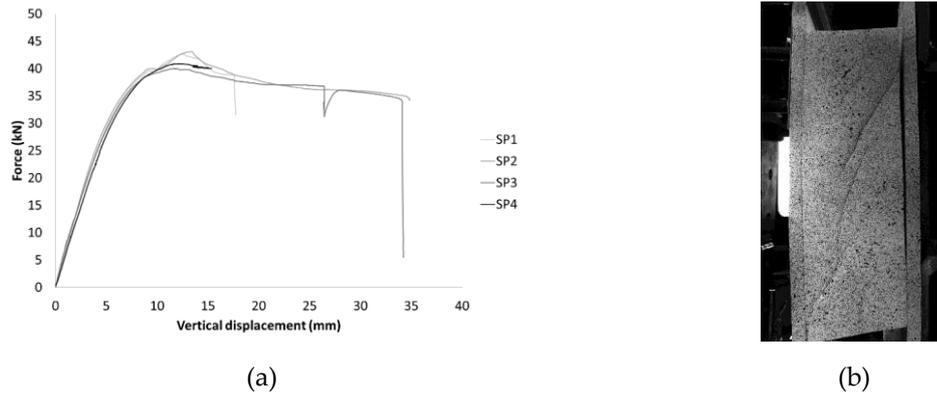
Figure 3. (a) force-displacement curve of the double-lap shear test, (b) picture of specimen at failure
