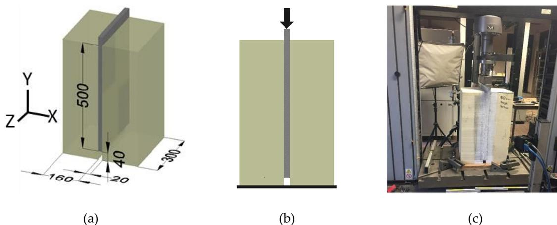
**Figure 2.** (a) specimen geometry with dimensions in mm, (b) schematic presentation of the test set-up, (c) picture of the test set-up
