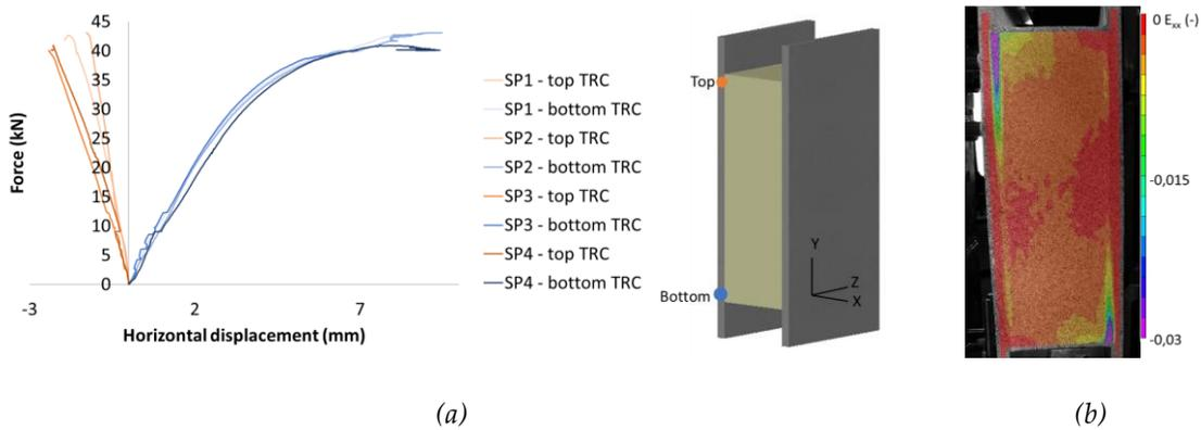
Figure 4. (a) horizontal displacement (x-direction) of the top and bottom of the loaded TRC face, (b) compression at the interface
