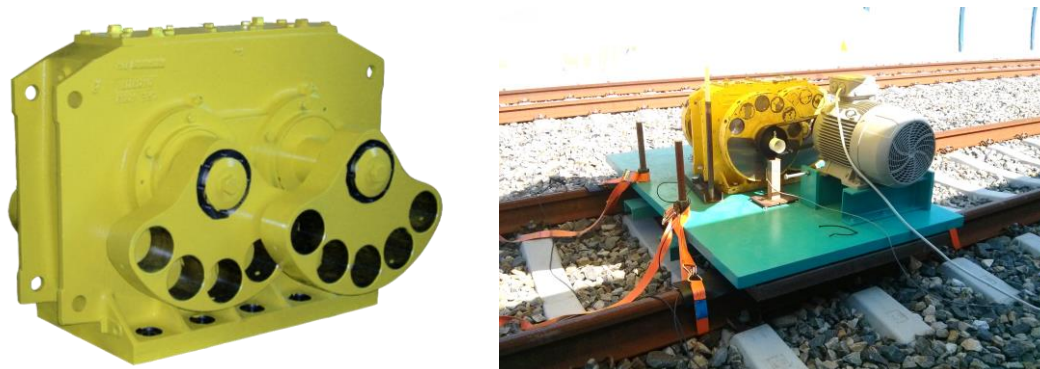
Figure 2. Unbalanced vibration exciter for experimental modal testing of railway bridges
