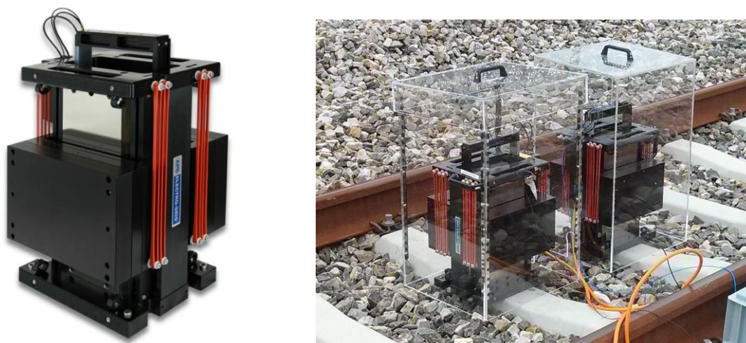
Figure 1. Electrodynamic long stroke shakers for experimental modal testing of railway bridges
