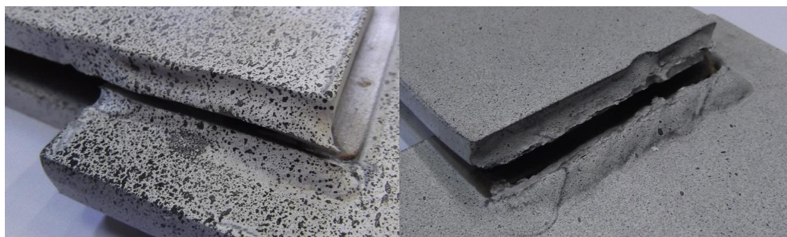
Fig. 2 Typical failure mode for longitudinal welds (left) and transverse welds (right).
