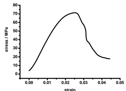
Fig.2 Static compression stress-strain curve of PBX simulation material
