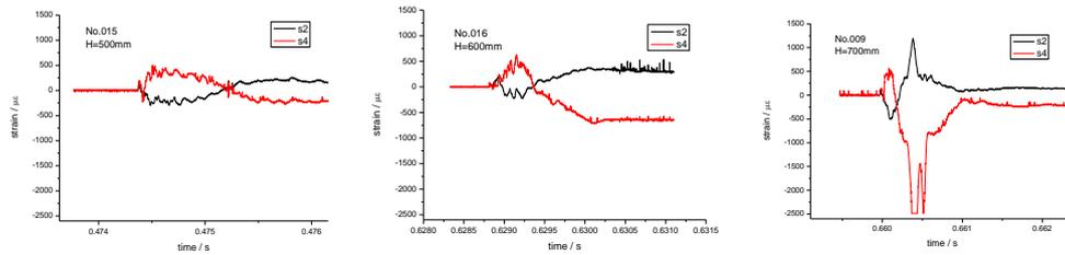
**Fig. 8** Strain of PBX simulation material surface during impact
