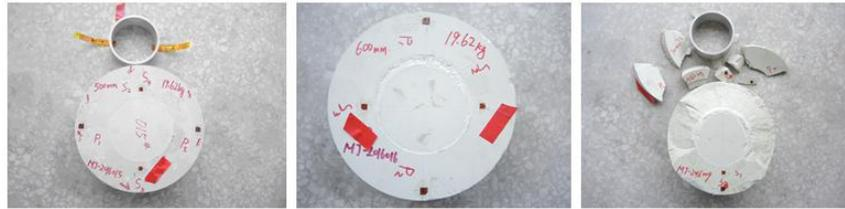
**Fig. 7** Morphology of PBX simulation material after drop test
