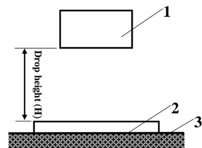
1. drop test piece; 2. target; 3. rigid base
