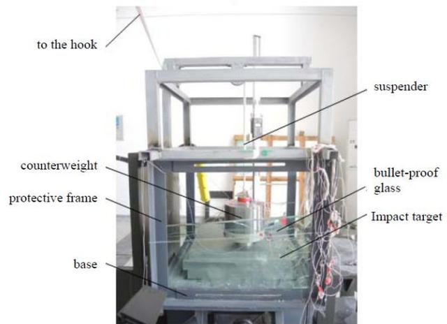
Fig. 5 Dropping test device
