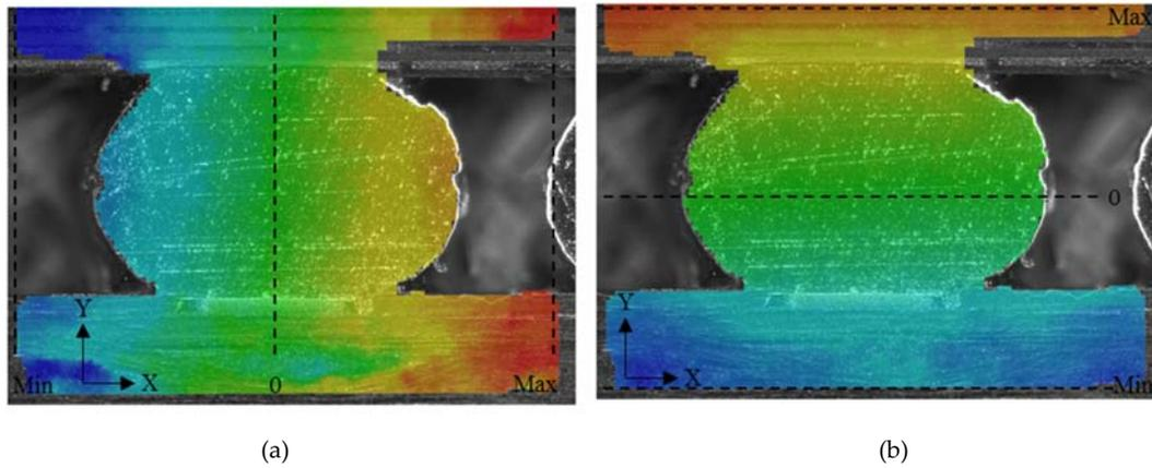
**Figure 3.** Relative Displacement at 170 °C in the (a) X-Direction and (b) Y-Direction at 200x Magnification
