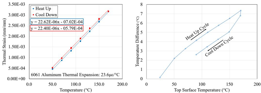
**Figure 4.** (a) Thermal Strain of the Aluminum as a Function of Top Surface Temperature and (b) the Temperature Difference Between the Top and Bottom Surfaces
