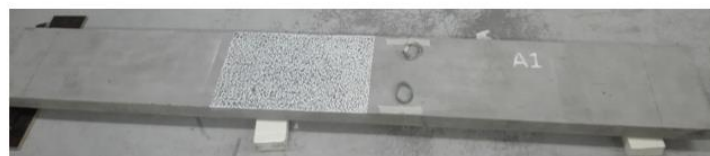
Slab A1: RC slab control specimen
