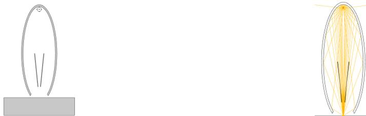
(a) Optimised geometry according to simulations. (b) Ray trajectories according to ray-tracing simulation.
