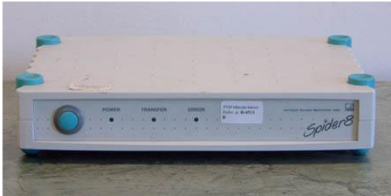
Figure 2. Spider 8, a strain gage measurement device
