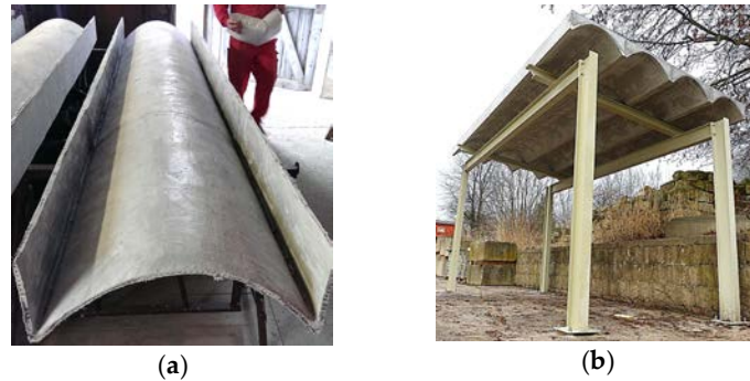
Figure 1. Ceiling element constructions: (a) a single, unfilled ceiling element (Photo: Tilo Senckpiel); (b) shelter consisting of four filled ceiling elements as demonstrator (Photo: Ludwig Pickert).
