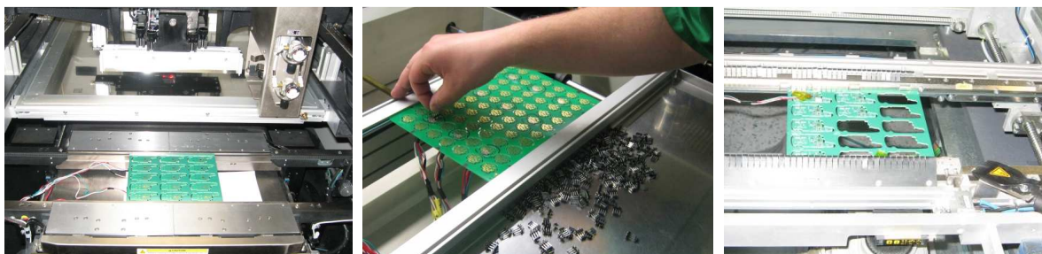
Figure 2. Solder paste printing, connector manual assembly and PCB depanelling
