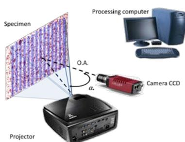
Figure. 1 Schematic set-up for FP+ 2D DIC Technique
