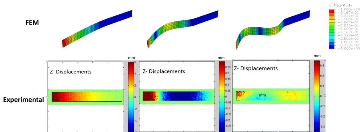
Figure 5 Modal test results of Finite element Method (left) and FP+2D-DIC technique (right).
