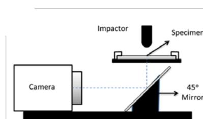
Figure. 2 Scheme of the experimental set-up for impact test on aluminium plate. .
