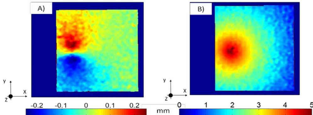
**Figure 4** (s) Y-Direction and (b) Z-Direction displacement maps occurring at maximum displacement instant during test.
