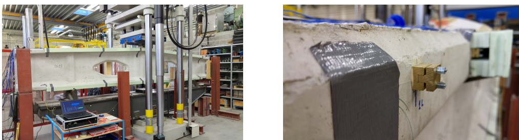
Figure 1. The experimental setup of the modal test. (a) Side view of the experimental setup. (b) One of the connections for the FBG sensors.
