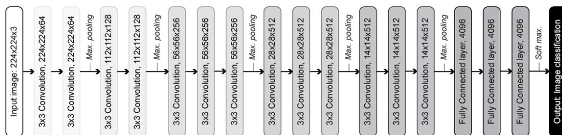
Figure 2. VGG16 architecture - the last layer was re-trained based on the transfer-learning approach.
