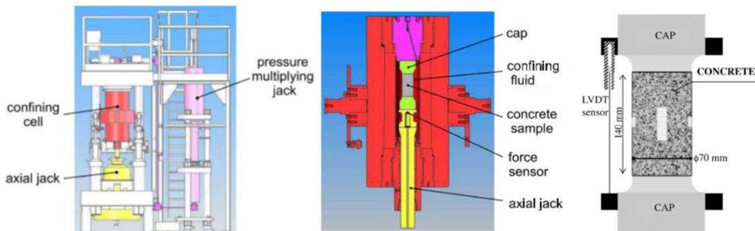
Figure 1: GIGA press (a) general view (b) section of the confining cell (c) sample instrumentation
