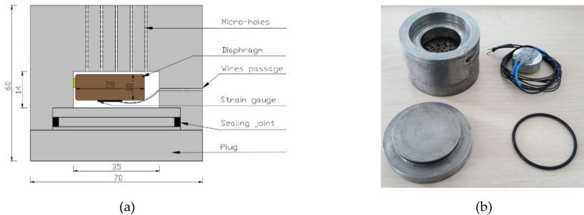
Figure 2: Water collecting cap with the sensor of hydrostatic type (a) design and (b) real concept
