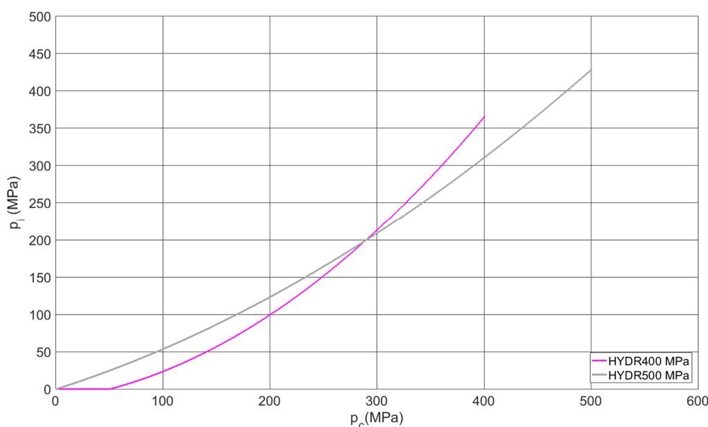
Figure 4: Pore pressure tests result: pore pressure  $p_i$  vs. confining pressure  $p_c$
