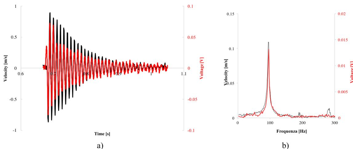
**Figure 6:** a) Comparison of the laser response and of the electrospun sensor; b) Fourier Transform with random fibers.
