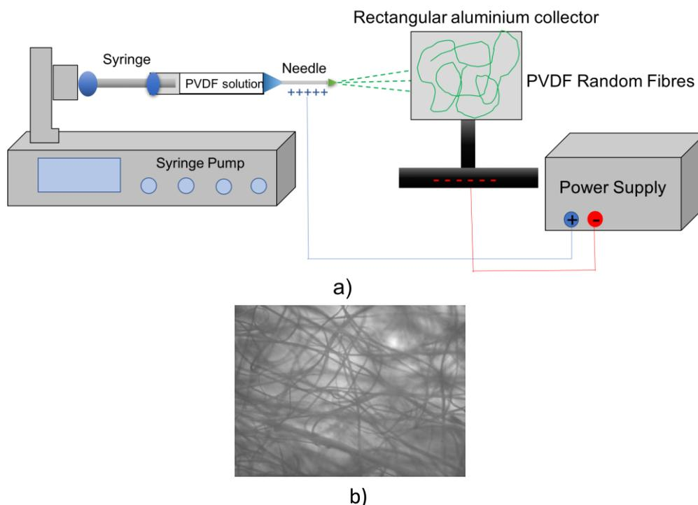
**Figure 1:** a) far field electrospinning setup; b) Microscope image of the PVDF porous mat formed by random fibers.
