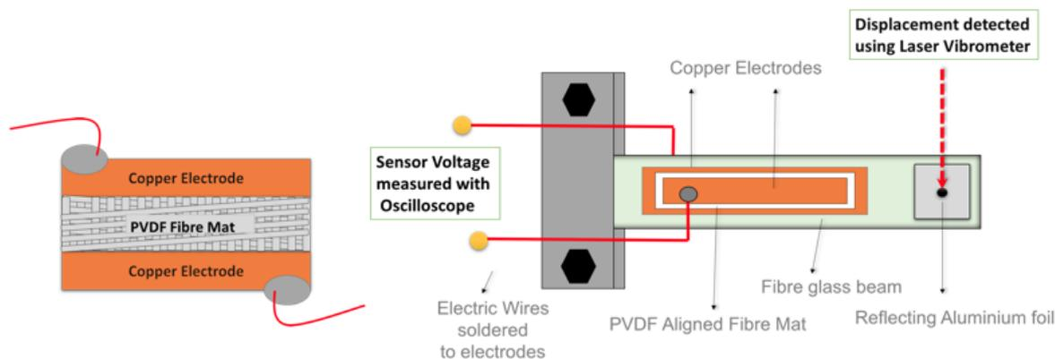
**Figure 5:** left side) schematic representation of the PVDF fiber mat sensor in the sandwich configuration; right side) Schematic representation of the sensing test setup.
