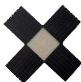
Figure 4: SMC composite biaxial specimen with continuously reinforced arms
