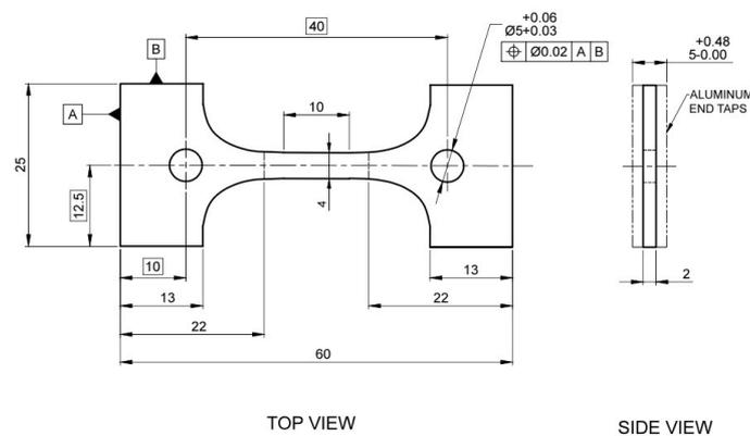
**Figure 1.** Tensile sample geometry
