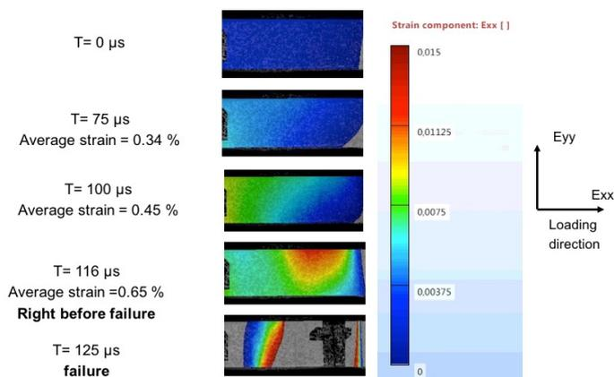
Figure 5. Full strain fields using 3D DIC
