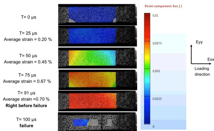
Figure 4. Full strain fields using 2D DIC
