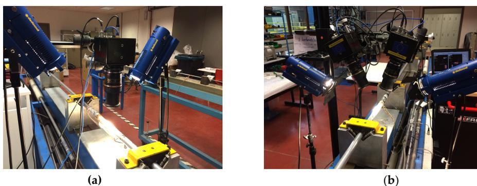
Figure 2. High speed DIC setups (a) 2D (b) 3D
