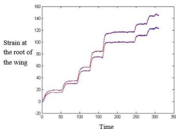
**Figure 7** Wind tunnel strain test results
