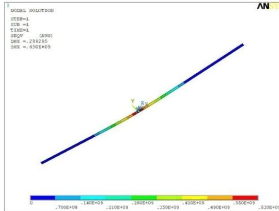
Figure 5 Stress of the wing of test model
