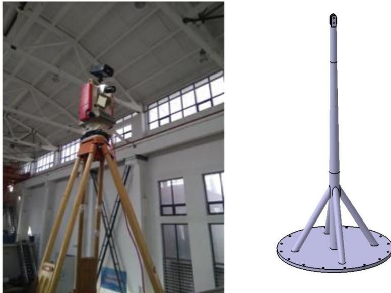
**Figure 1** Optical deformation measurement device and Ventral support device
