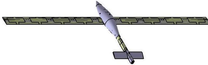
**Figure 2 Wind tunnel test model**
