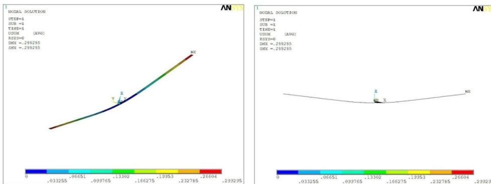
**Figure 4 Deformation of the wing of test model**
