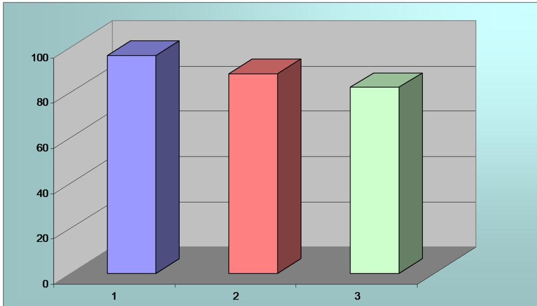
**Figure 7.** Recovery (in wt%) of La, Ce and Nd after magnetic separation ( sample No .123).
