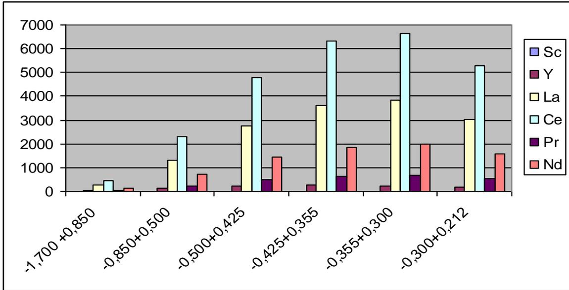
**Figure 6.** Distribution of LREEs in the magnetic fractions of the different grain sizes in the composite sample (Amixed).
