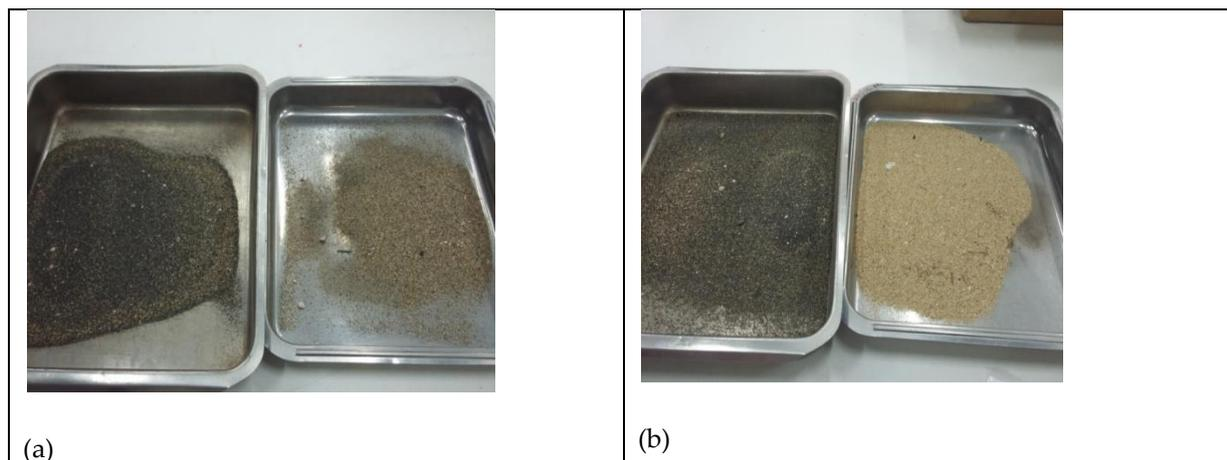
**Figure A1.** Photos of magnetic separation products. (a) First stage separation of the magnetic and non magnetic product (b) Second stage separation of the magnetic product.
