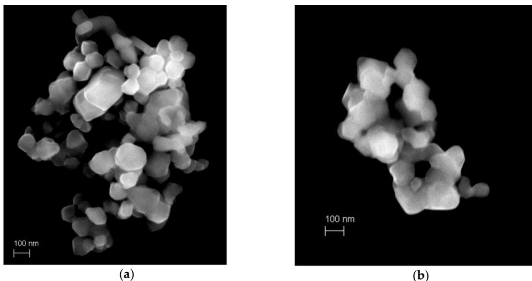
132 **Figure 2.** The SEM pattern of the 1.25 NCM(a) and 1.20 NCM(b)
