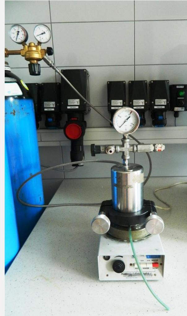
Fig. 2. The steel filter cell for membrane filtration
