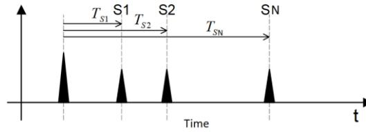
**Figure 1.** Schematic visualization of acoustic arrival times on a set of sensors (S1, S2, ..., SN)[7].
