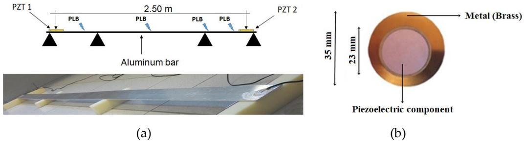
**Figure 2.** (a) Experimental Setup and (b) piezoelectric diaphragm.
