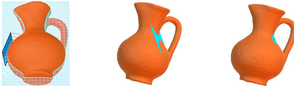
Figure 3. Adaptive modification of tactile sensor size.
