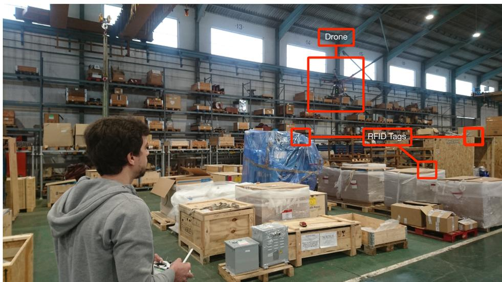
Figure 4. One of the instants during the inventory tests.
