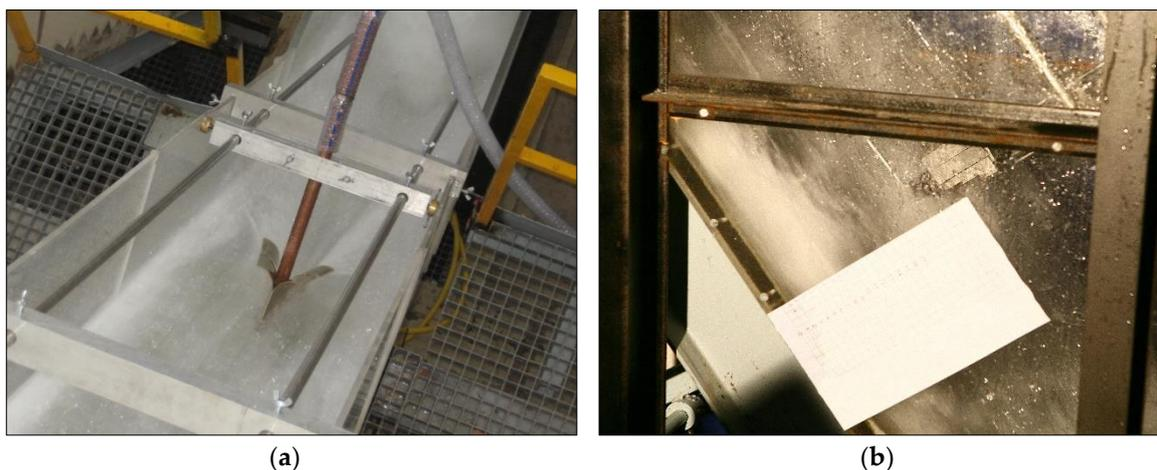
123 **Figure 5 (a):** Pitot probe during the velocity measurement process. **(b):** ACM during the concentration
