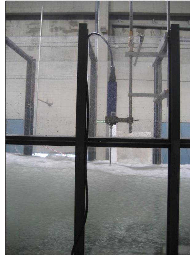
Figure 26. ADV probe velocity test in hydraulic jump
