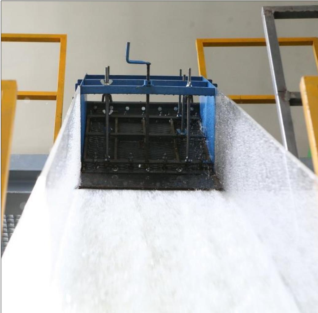
Figure 4. Intake flow section gate
