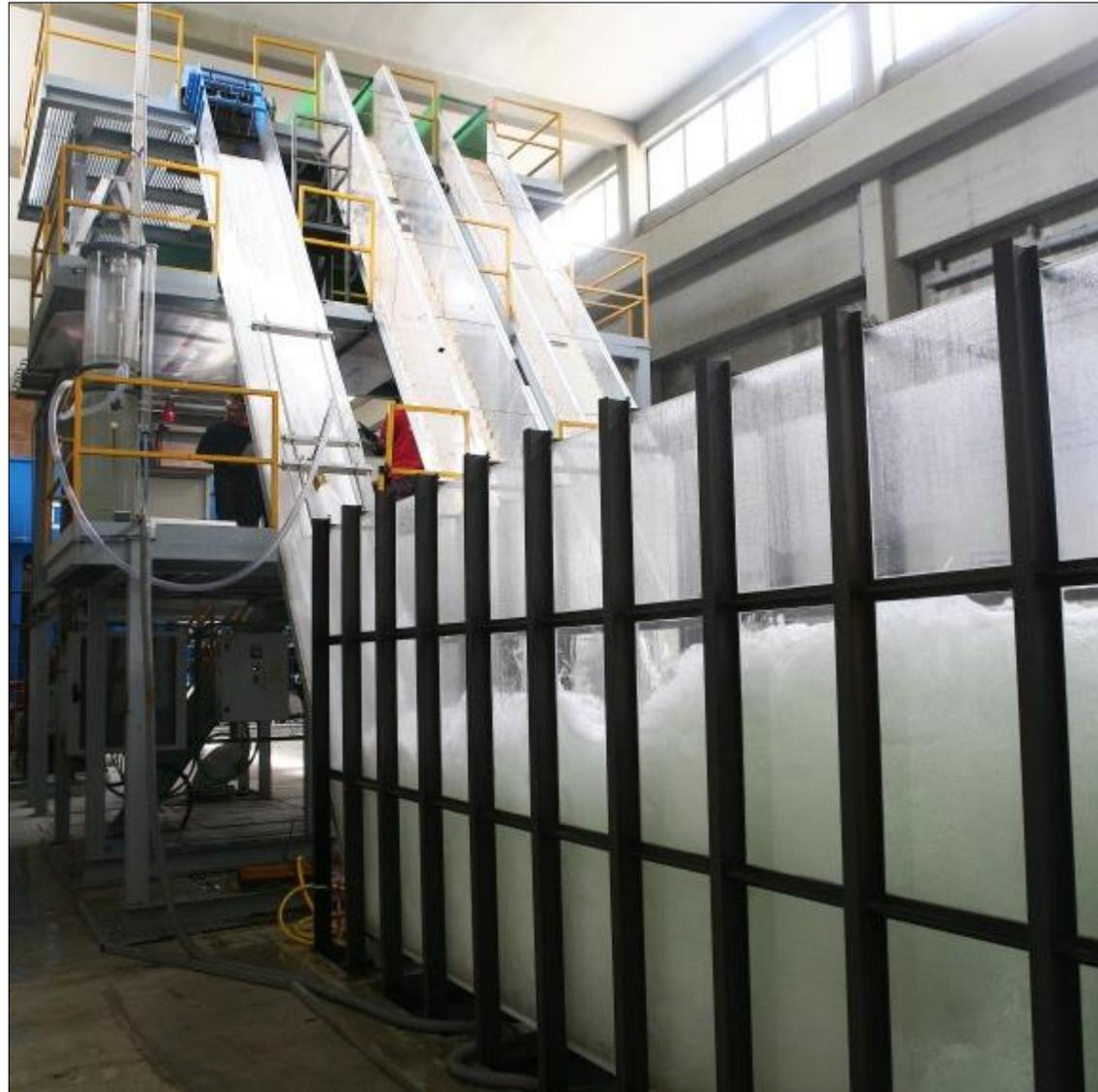
Figure 3. Global view of physical model with spillway and still basin
