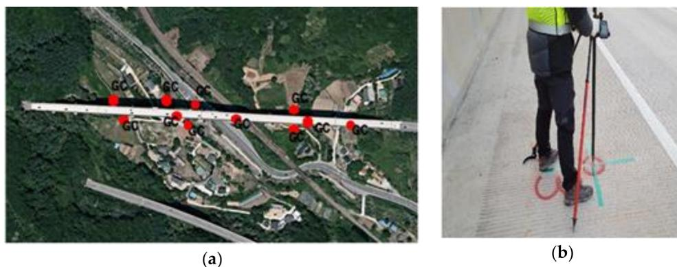
Figure 1. Wonjudaegyo Bridge, Korea: (a) Aerial view with control point locations; (b) Installation of control points before flying UAV.
