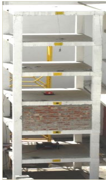
Figure 1. RC building Frame with Masonry Infill.
