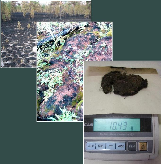
On-ground cover pattern after burning / Measurement of amount of on-ground cover after burning
