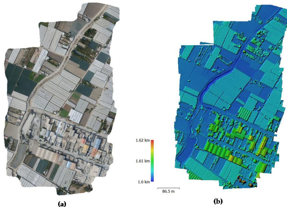
Figure 5. Products generated by the SVAID. (a) orthomosaic, and (b) DSM.
