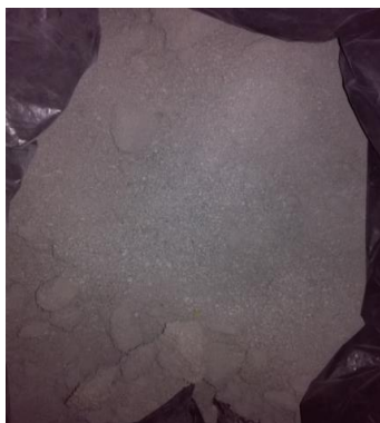
Figure 1. Air dried tannery sludge obtained from the respective wastewater treatment plant.
