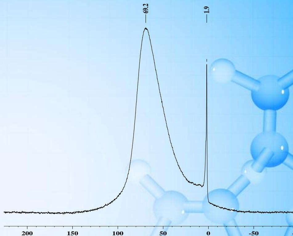
In  $^{27}\text{Al}$  NMR spectra of the diluted solutions in  $\text{CDCl}_3$  very intensive signal of 40.0–90.0 ppm (4-coordinated) and weak signal of 0.0–5.0 ppm (6-coordinated) are observed. This, apparently, is related to a rupture of coordination bonds between the aluminum atom and carbonyl groups
