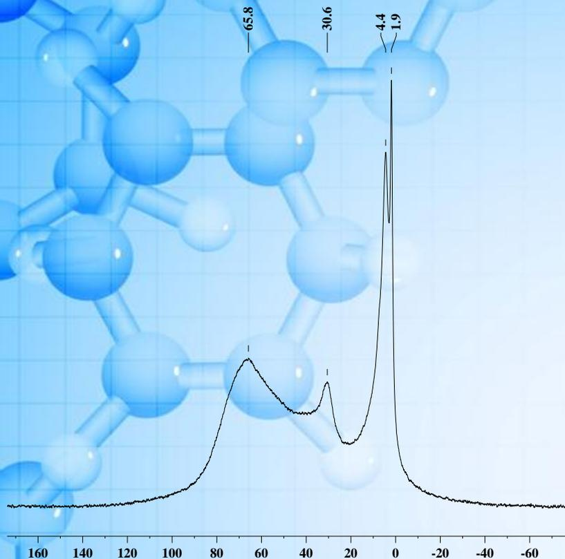
In  $^{27}\text{Al}$  NMR spectra (600.13 MHz,  $\text{CDCl}_3$ ) of the concentrated oligomer solutions in  $\text{CDCl}_3$  three types of signals of almost the same intensity are recorded: 70.0–80.0 ppm (4-coordinated), 30.0–45.0 (5-coordinated), 1.8–7.5 ppm (6-coordinated).
