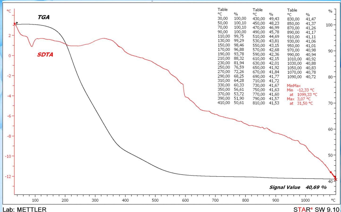
The TGA curve shows that the oligomer is stable when heated to a temperature of  $\approx 200$  °C. The main weight loss occurs in the temperature range of 200–500 °C (the remainder is about 45 weight %). Further, the removal of residual hydroxyl groups in the form of H<sub>2</sub>O vapor is observed, the ceramic residue is 40.69 wt %, which corresponds to the theoretical values (slide 6).
