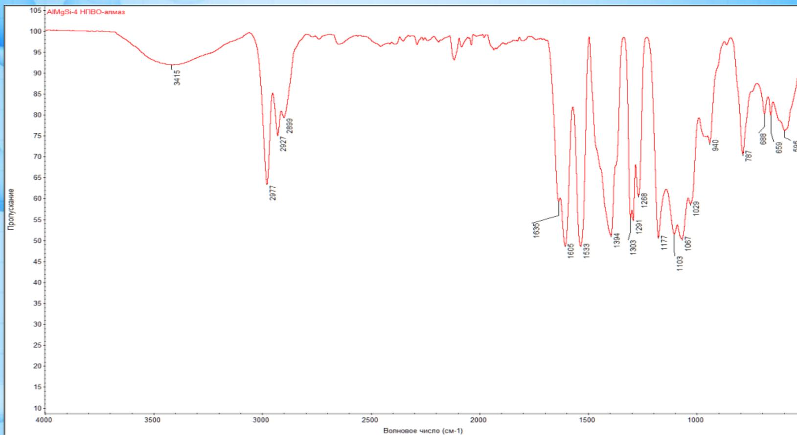
IR (cm<sup>-1</sup>): 595  $\nu$ (Mg–O–Al), 659, 688  $\nu$ (Mg–O; Al–O; Si–O), 863  $\nu$ (Al–O–Al), 940  $\nu$ (Mg–O), 967  $\nu$ (Al–O<sub>4</sub>; Si–O), 1030, 1071, 1101, 1176  $\nu$ (Mg–O–C; Al–O–C; Si–O–C), 787, 1268, 1291, 1303, 1398  $\delta$ {CH, C(CH<sub>3</sub>)} and  $\nu$ (C–O), 1533  $\nu$ (C=C), 1602  $\nu$ (C=O from [CH<sub>3</sub>(O)CCH=C(CH<sub>3</sub>)O]), 1635  $\nu$ (C=O, bonded by coordination bond with Al atom), 2899, 2927, 2977  $\nu$ (CH), 3415  $\nu$ (OH)
