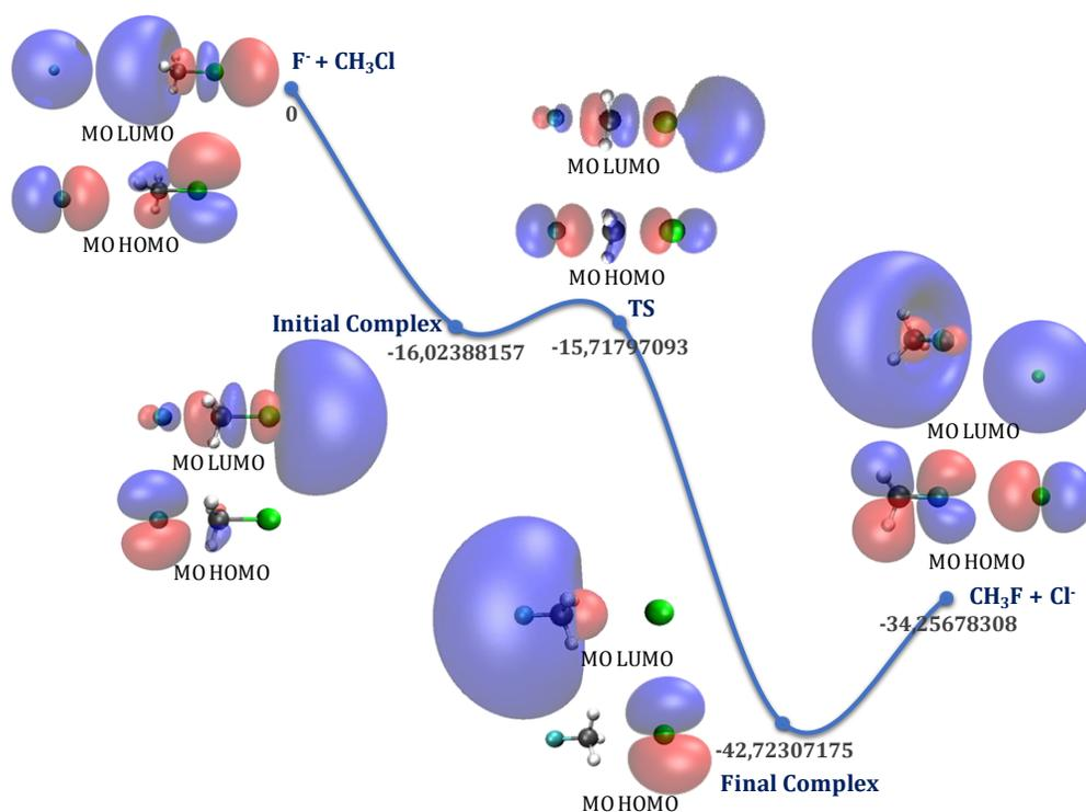
**Figure 6.** MOs HOMO and MOs LUMO for the stationary points at PES for the S<sub>N</sub>2 reaction of F<sup>-</sup> and CH<sub>3</sub>Cl in the gas phase
