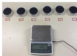
Figure 5. Verification aliquots of pellet feed standard samples after weighing and heating for 24 hours at 105°C.
