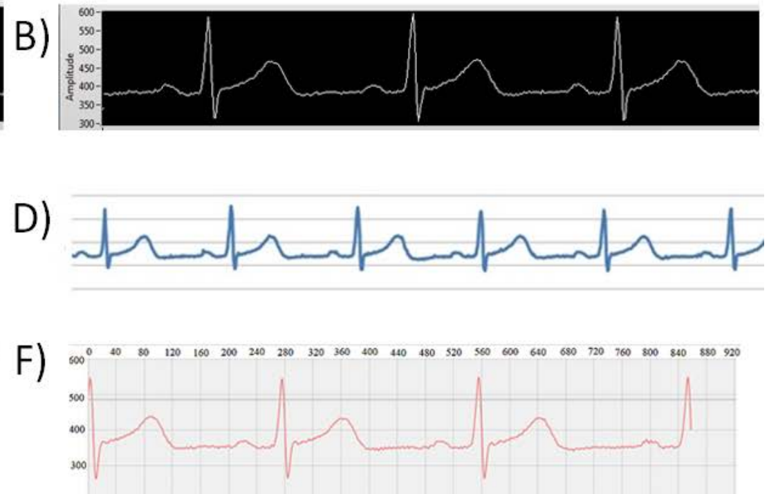
Figure 22. Snapshots of different operation modes. A) ECG signal transmitted by serial cable (breadboard prototype), B) ECG signal transmitted by serial cable (custom PCB), C) ECG recorded to a microSD card (breadboard prototype), D) ECG recorded to a microSD card (custom PCB), E) ECG signal transmitted by Bluetooth via smartphone (breadboard prototype), F) ECG signal transmitted by Bluetooth via smartphone (custom PCB). The sampling frequency in all signals was 360 Hz.
