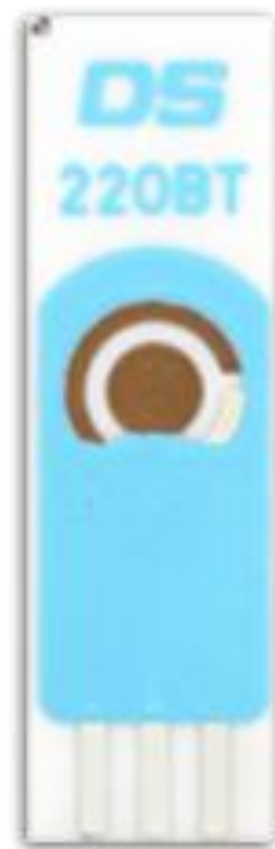
Au/SPE low temperature cure ink gold electrode; E_w (4 mm diameter)
