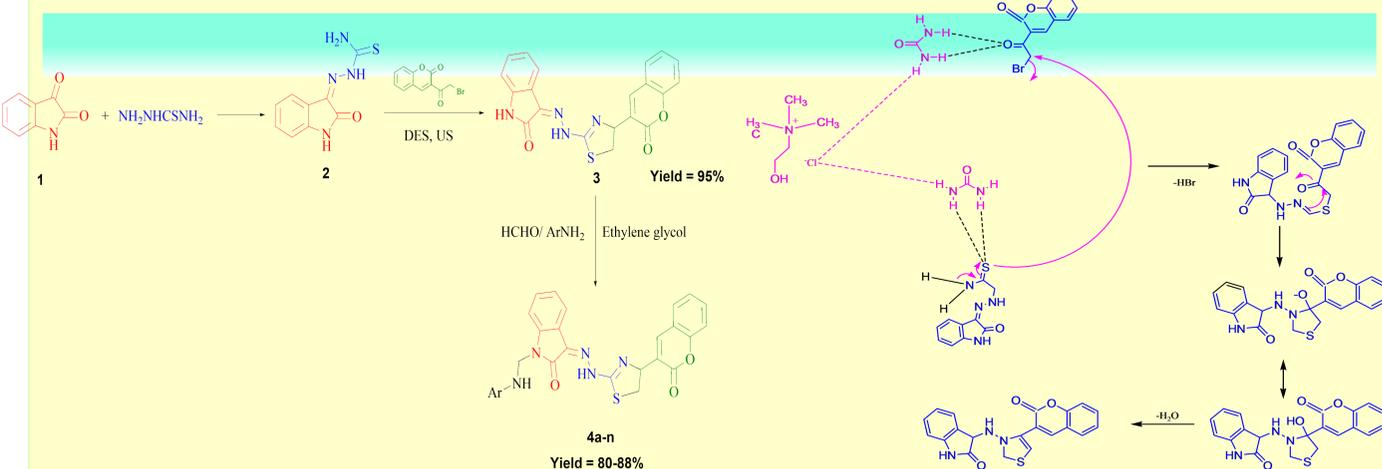
**Scheme 2.** Schematic representation of synthesis of compounds (4a-n) via key intermediate (3) isolated from deep eutectic solvent and ultrasound blend of technique.
