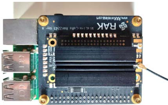
Figure 2. RAK2245 module with a RaspBerry Pi board
