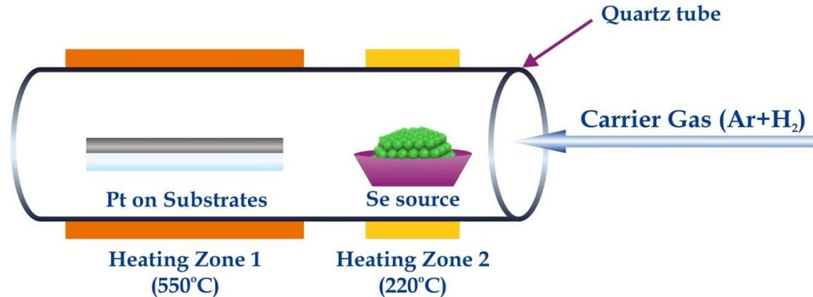
Fig. CVD selenization process
