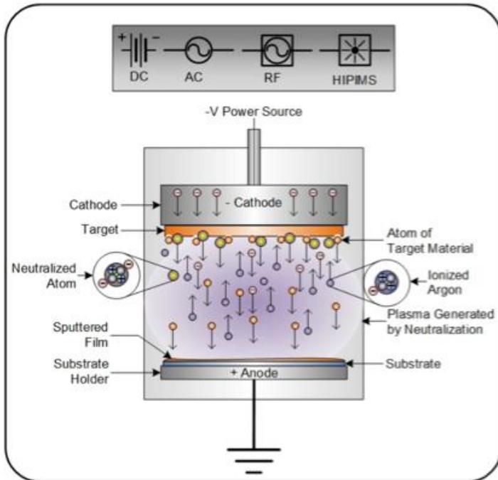
Fig. Magnetron sputtering
