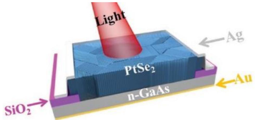
*Fig. Schematic illustration of  $PtSe_2/GaAs$  heterojunction based photodetector*
