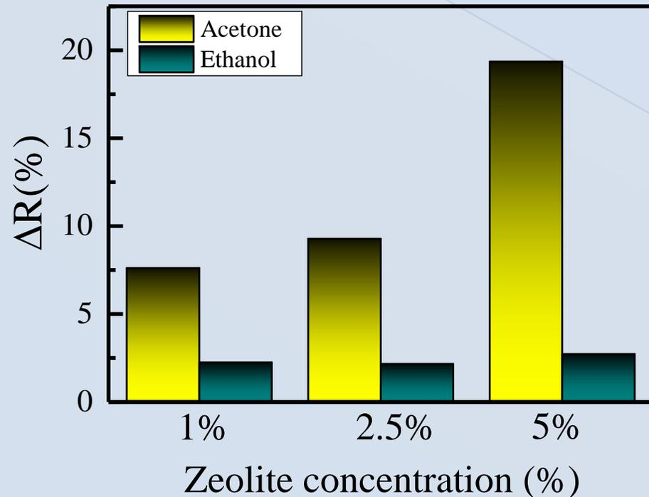
Zeolite concentration dependence of reflectance change induced by exposure to liquid acetone (yellow) and ethanol (green) of milled zeolites embedded in thin  $\text{Nb}_2\text{O}_5$  films. Measurements are conducted at room temperature.
