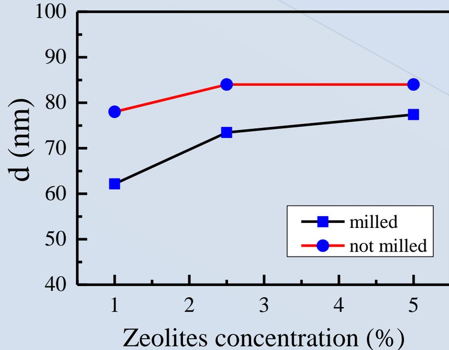
Dependence of thickness  $d$  on zeolite concentration (b) of thin  $\text{Nb}_2\text{O}_5$  films embedded with not-milled and milled fly ash FAU zeolites.
