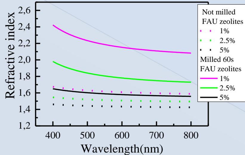
Dispersion curves of refractive index of thin Nb<sub>2</sub>O<sub>5</sub> films embedded with not-milled and milled fly ash FAU zeolites.
