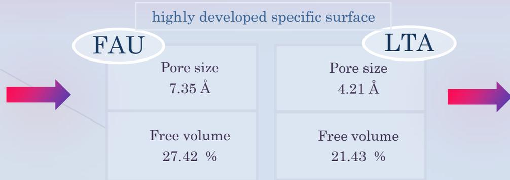
Allowing the physical adsorption of molecules of CO<sub>2</sub> from size 3.2 Å
