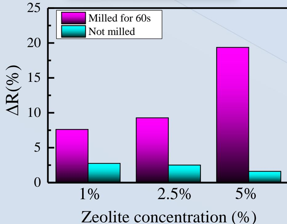
Zeolite concentration dependence of reflectance change induced by exposure to liquid acetone of FAU not-milled (blue bars) and milled (magenta bars) embedded in thin  $\text{Nb}_2\text{O}_5$  films. Measurements are conducted at room temperature.
