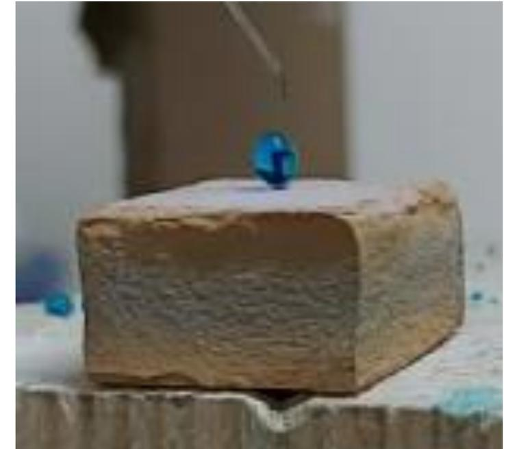
The no reported results correspond to samples which the water droplet bounces off the surface, characteristic of superhydrophobic behavior.
