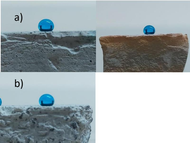
Water droplets over coated surfaces (left concrete, right clay) a) 10 layers, b) 15 layers
