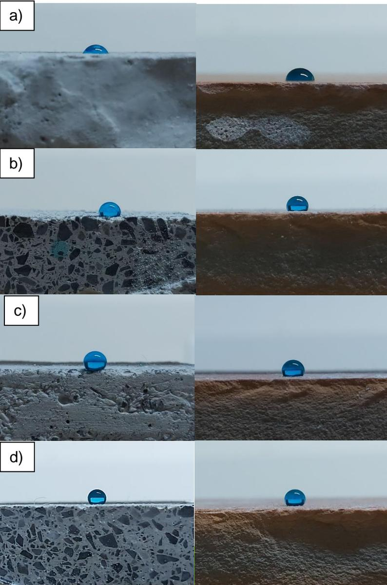
*Water droplets over coated surfaces (left concrete, right clay) a) control, b) 10 layers, c) 15 layers d) 20 layers*
