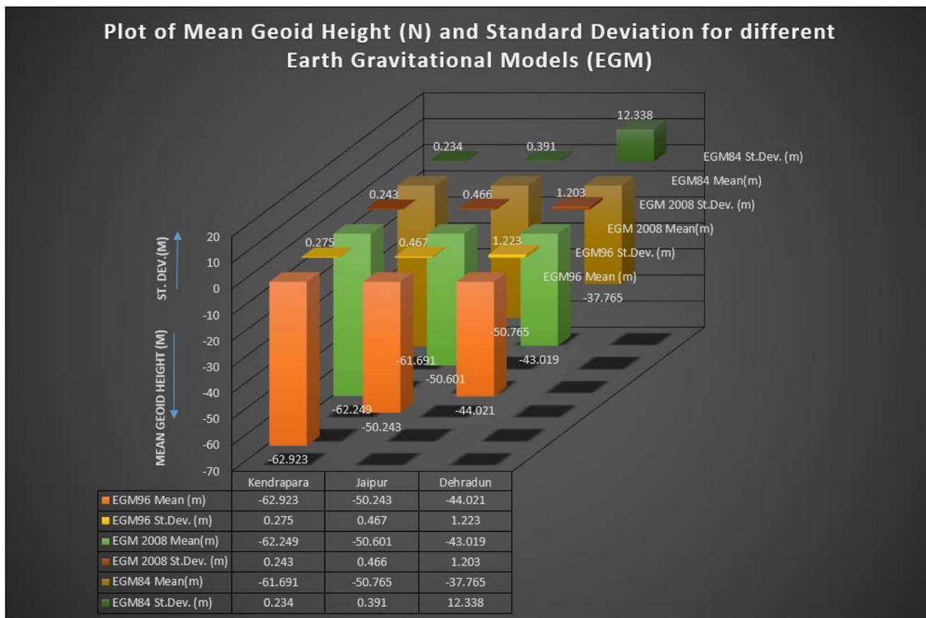
**Figure 2:** Plot of Mean Geoid Height (N) and St. Dev. for different Earth Gravitational Models (EGM)
