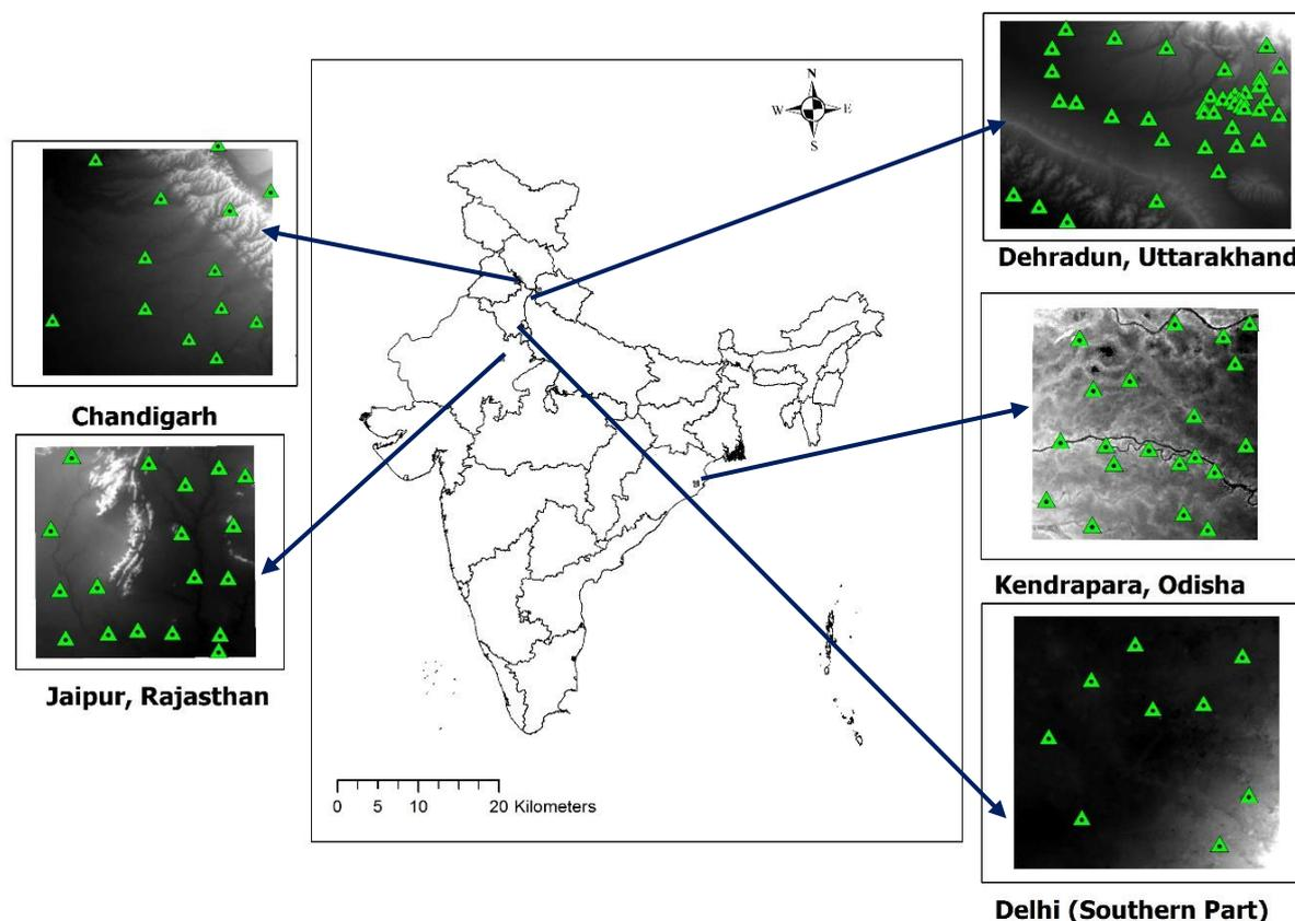
**Figure 4:** Location map depicting DEMs of experimental sites with overlaid GCPs collected using Differential GPS survey
