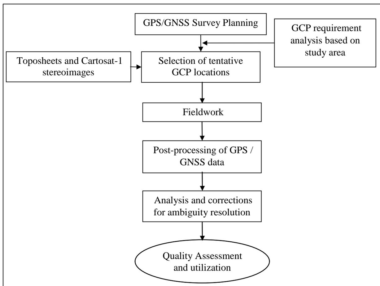
**Figure 1:** Methodology for Differential GPS / GNSS survey
