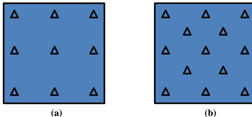
**Figure 2:** Depicts ideally planned scheme for distribution of GCPs for conducting GNSS survey (a) plan indicates von-Grubber location and (b) plan represents further
