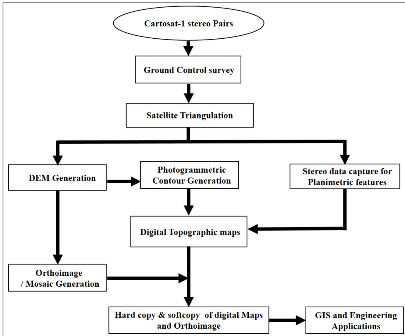
Figure 3: Methodology for Photogrammetric procedure
