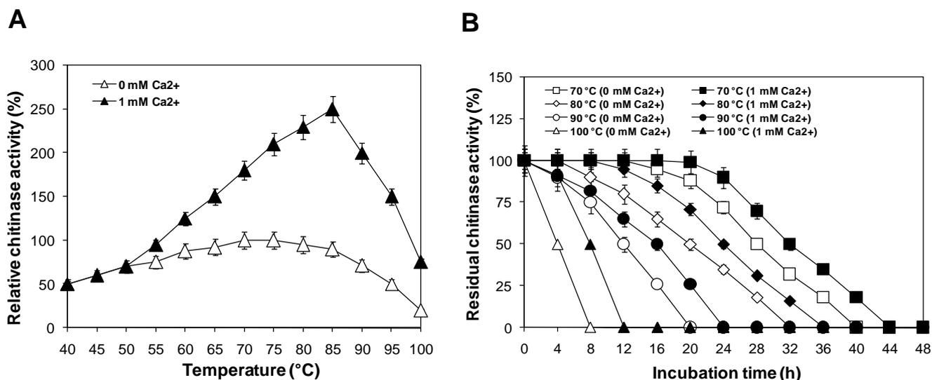
**Fig. 3.** Effect of the thermoactivity (A) and the thermostability (B) of ChiA-Ba43. Each point represents the mean of at least three independent experiments.
