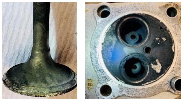
Figure 9. Deposit formation on engine parts.
