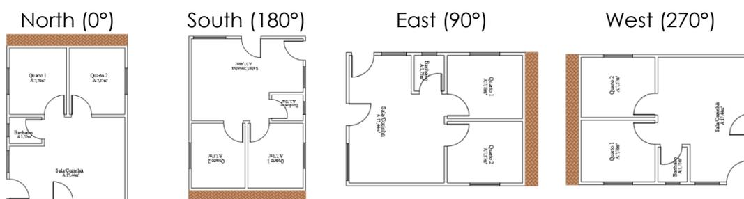
**Figure 4.** Variation of the embedded earth-sheltered wall orientation.
