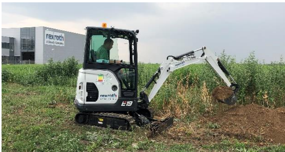
Figure 19. The electric excavator E19 when digging.
