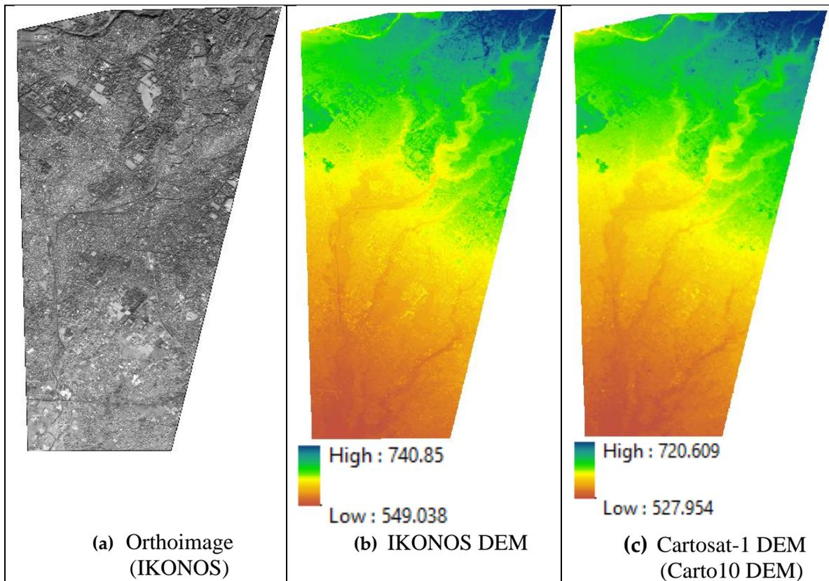
164 **Figure 5.** (a) Orthoimage for the reference DEM site, Comparison of (b) reference data (IKONOS
