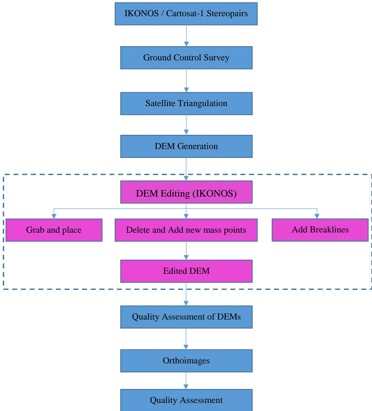
142 **Figure 4.** Photogrammetric methodology used for satellite triangulation, DEM and orthoimage
