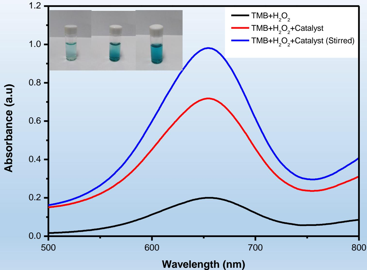
UV-vis spectra for TMB oxidation with H<sub>2</sub>O<sub>2</sub> without nanozyme (black), with nanozyme (red), and with nanozyme on a magnetic field (blue) (Inset picture: TMB+H<sub>2</sub>O<sub>2</sub> (left), TMB +H<sub>2</sub>O<sub>2</sub>+Nanozyme (middle), and TMB +H<sub>2</sub>O<sub>2</sub> + Nanozyme (on magnetic field) (right))
