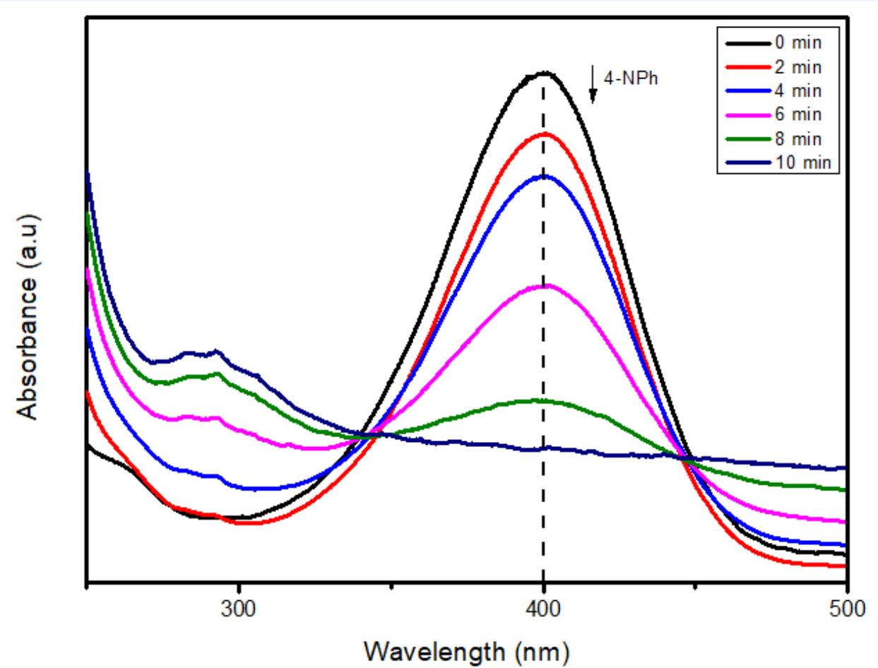
UV-vis spectra for a) Non-magnetic field-assisted reduction of 4-nitrophenol
