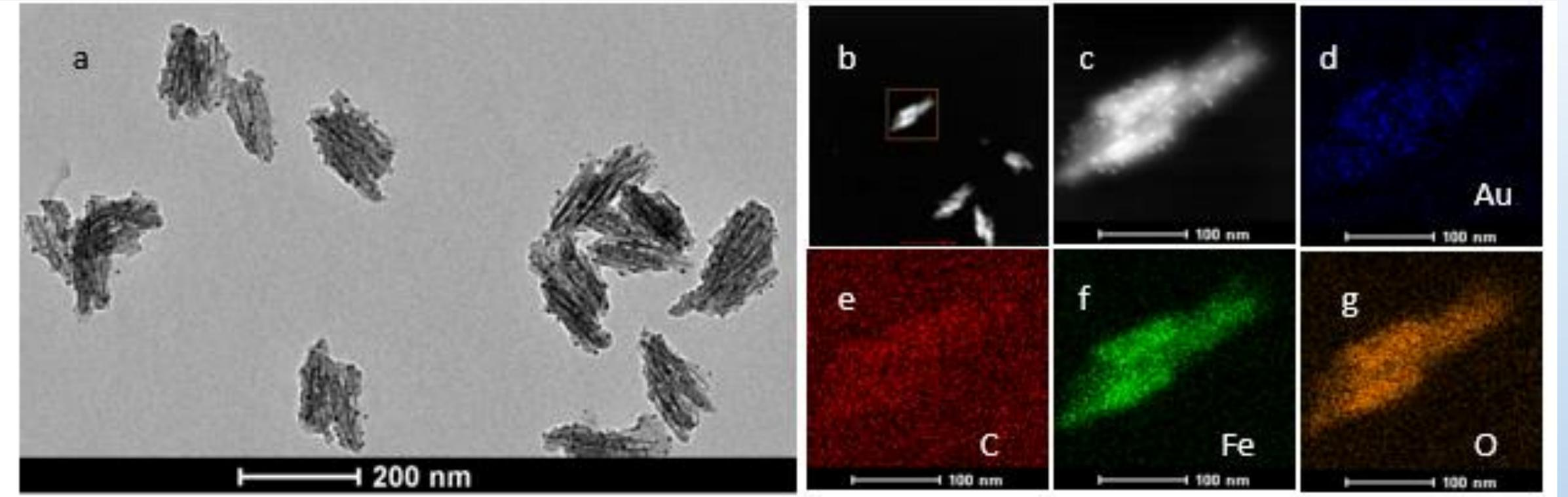
a) TEM image of  $\text{Fe}_3\text{O}_4@MIL-100(\text{Fe})-\text{Au}$ ; b, c) STEM HAADF image of composite; Corresponding elemental analysis results d) Au; e) C; f) Fe and g) O
